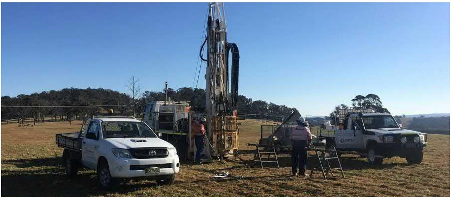
Fig 2: Typical setup for a geotechnical investigation
